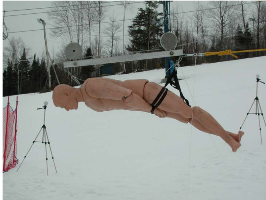
Fig. 1 Photograph illustrating the test apparatus set-up for head first impact
