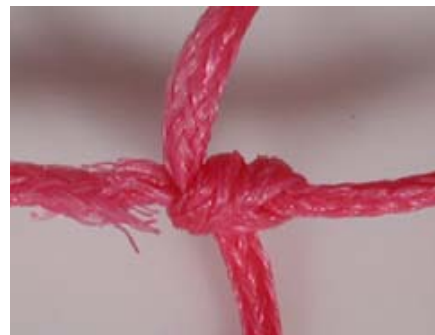
Knotted polyethylene breakdown after exposure to 500 hrs QUV, and prior to being tested for residual tensile strength.
