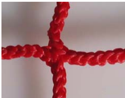
Knotless nylon netting showing no evidence of breakdown after exposure to 500 hrs QUV, and prior to being tested for residual tensile strength.
