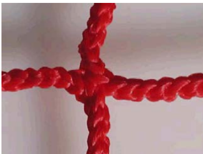
Nylon netting showing no evidence of breakdown after exposure to 500 hrs UV, and prior to being tested for residual tensile strength.
