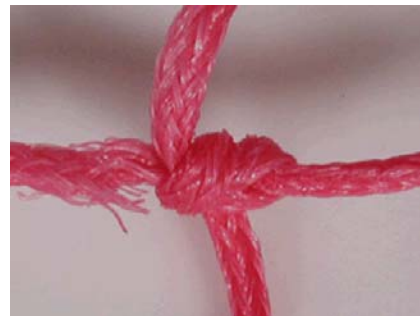
Knotted polyethylene breakdown after exposure to 500 hrs UV, and prior to being tested for residual tensile strength.
