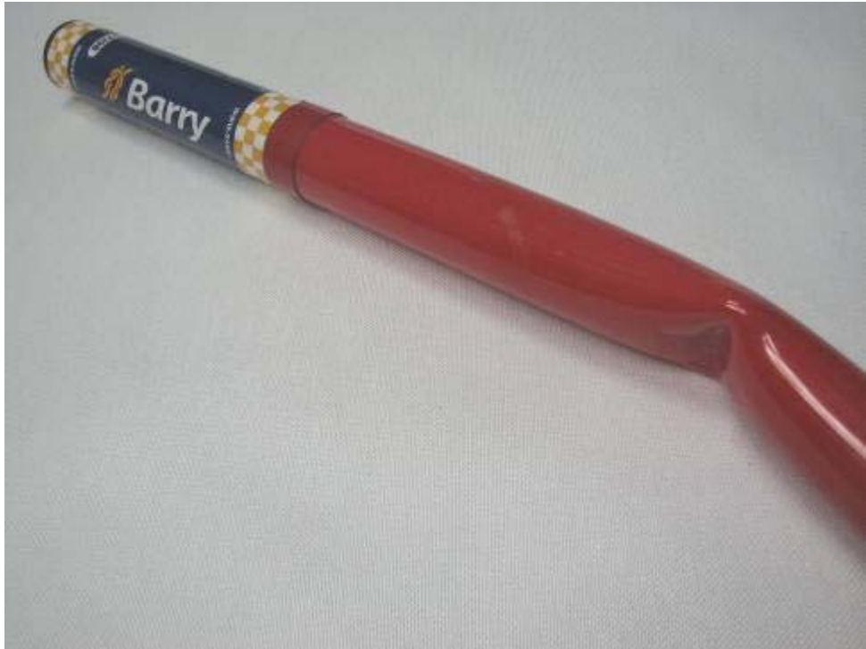
Photo 7: Showing ductile bend
