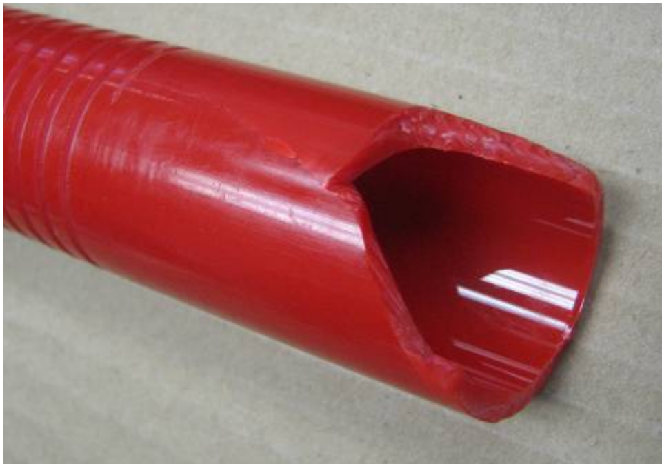
Photo 4: Detail view of fractured end
