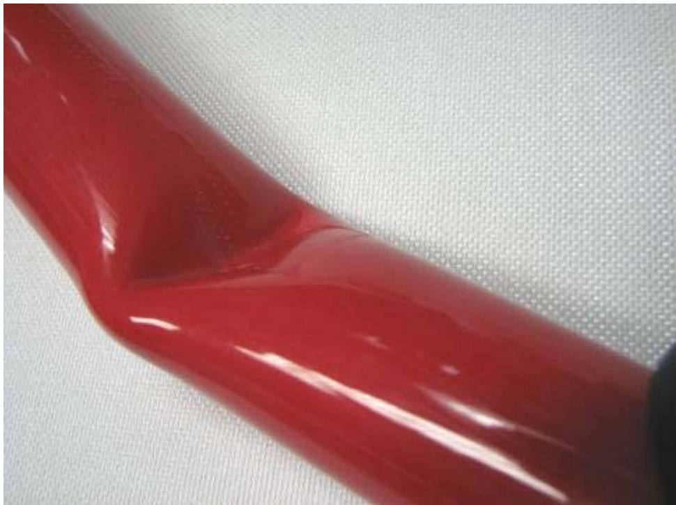
Photo 8: Detail view showing ductile bend
