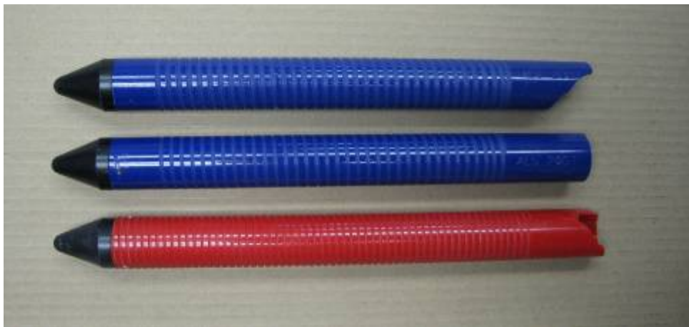
Photo 1: Showing the bases of the broken scribed poles
